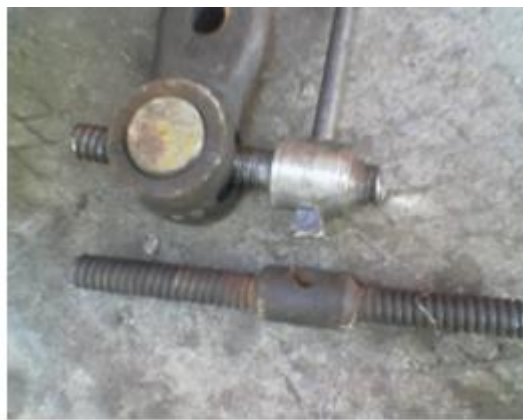
Fig:- 1.2 photograph of broken coupler screw
